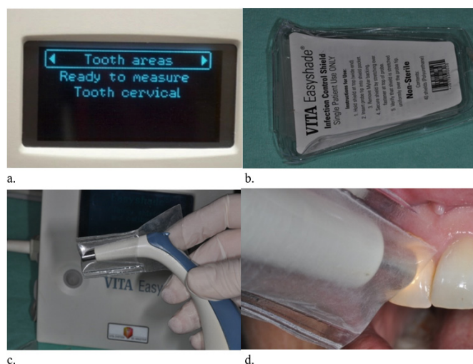
Fig. 1. a. Program Tooth Areas of the spectrophotometer Vita Easyshade®; b. Infection control shield; c. The infection control shield placed on the probe tip; d. Digital measuring of the tooth color.
