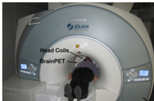
Fig. 2. Siemens MR-BrainPET prototype (PET insert into an MR scanner). (15)
