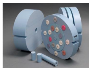
Fig.3. Presentation of the CIRS phantom with materials of different densities.
